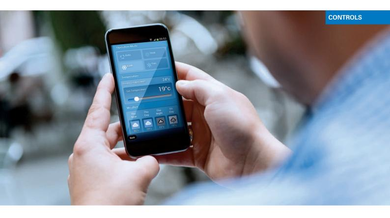
The MAC-567IF provides remote cloud control and monitoring over M series, Mr Slim, City Multi and Ecodan FTC5 series indoor units.
