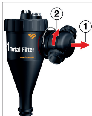
2. Pull the inlet/outlet port approximately 3 mm away from the body to allow rotation to the required position.
