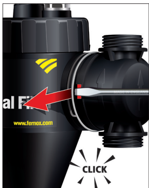
1. Using a flat end screwdriver in the recess shown, gently lever the locking clip into the 'unlock' position.
